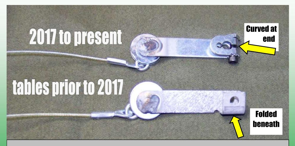
In 2017, tired of getting complaints about sheared ball drop motor shafts on bill-acceptor pool tables, we began using a ball drop motor with a sturdier shaft. The side-effect was this meant we needed to change the cable to accommodate the new shaft—and they're not interchangeable.
