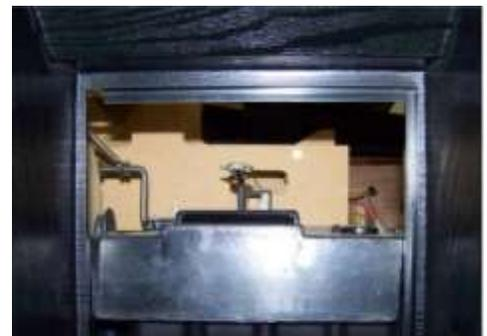
The current parts will cost several hundred dollars and will just not be a cost-effective solution on a 30 (or more) year old table. You will notice from the photo the door on the left is not as tall, but wider. You cannot adapt the current parts to fit in an older table because the original hole will be too tall, and you’ll have to widen it. We **STRONGLY RECOMMEND** you do not attempt this “upgrade.”
