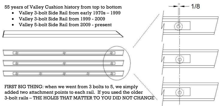
SECOND BIG THING: the change in 1999 moved 4 of the 18 bolt holes used to attach the rails by exactly 1/8". THAT is the difference between "old Valley" and "new Valley" – 1/8". Literally so close it wasn't physically possible to put in two inserts side-by-side.
