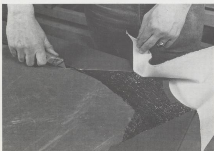
8 Cut the cloth diagonally back from the pockets with a utility knife.
