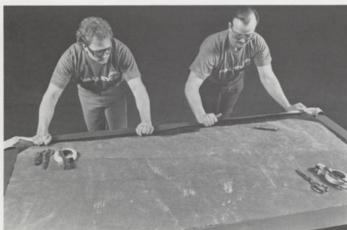
7 Move to the opposite side of the slate and lift while pulling the cloth tightly, then fold the cloth into the adhesive.
