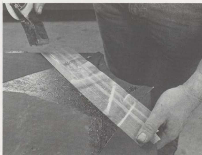
11 Pull the cloth tabs tightly around the slate and fold them into the adhesive as shown. Tape over the cloth tabs at each pocket to guarantee a tight hold. (Note: As the cloth tabs are pulled around the slate some tearing of the cloth at the cut lines may occur.) Your slate is now ready to reinstall back into your Valley table.
