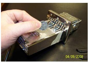
2) To gain access to the inserts, put your coins into the correct slots and then push in the handle.
