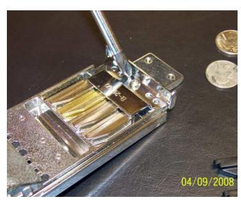
6) Regardless of if you have a V-4, V-5 or V-8 unit, the insert retainer plate holds the inserts in. Remove the Phillips screw or screws holding this plate and you will have access to all the inserts.
