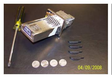
1) Remove the Push Chute from the coin door for easier access. You will need the Push Chute (of course), enough coins to make it work in its current setting, the inserts for the desired setting, and a Phillips screwdriver.
